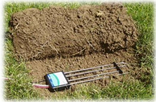
A soil moisture sensor, buried in the turf root zone prevents irrigation
