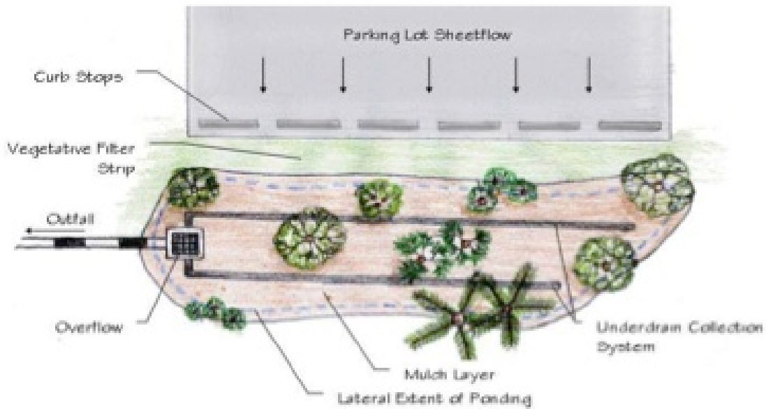
Figure 5.16.2. Cross Section View of a Biofiltration System
