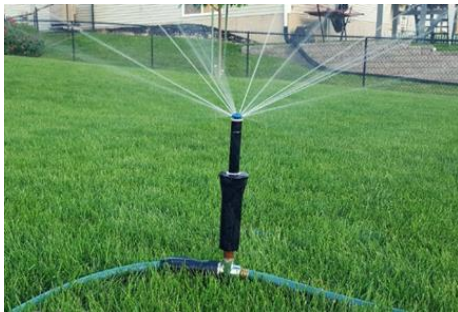
MP rotator attachment built with standard irrigation components.
