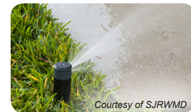
Without proper maintenance, spray heads can become too low to the ground to be effective.
