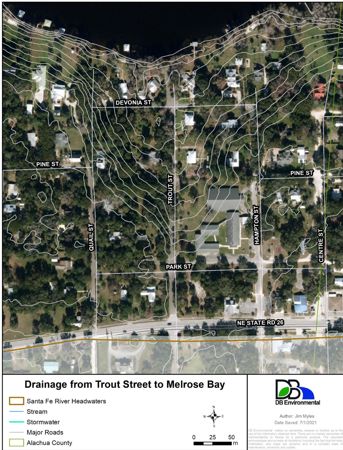
Figure 55. Stormwater runoff from Trout Street to Melrose Bay near the boat ramp.
