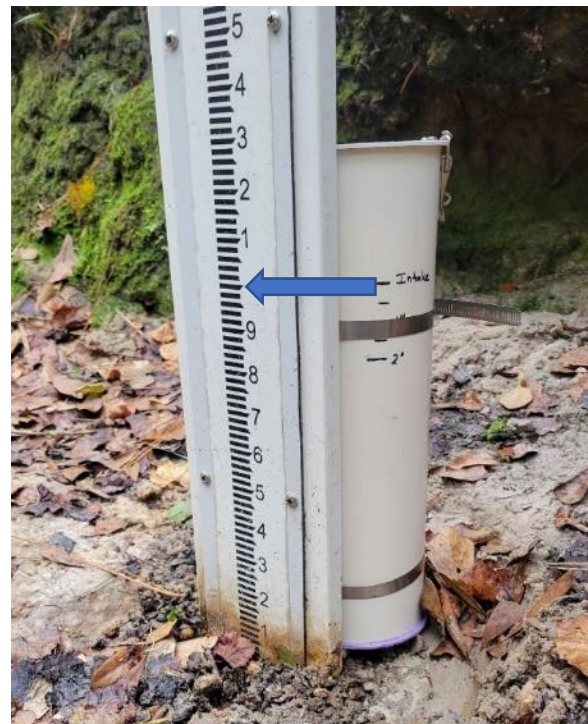
Figure 20. First flush sampler installed at the staff gauge in the southern culvert at NE 221 st Street.
